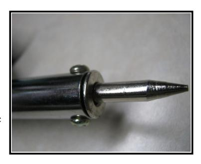
NEVER use you good iron or station for wood burning or plastic melting. Residue from those projects stays on you tip and fouls it for soldering!
