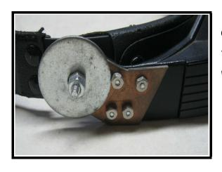
Fender washer & bolt for the hinge and a piece of copper clad pcb stock for a broken side piece and they work as good as they did 30+ years ago!
